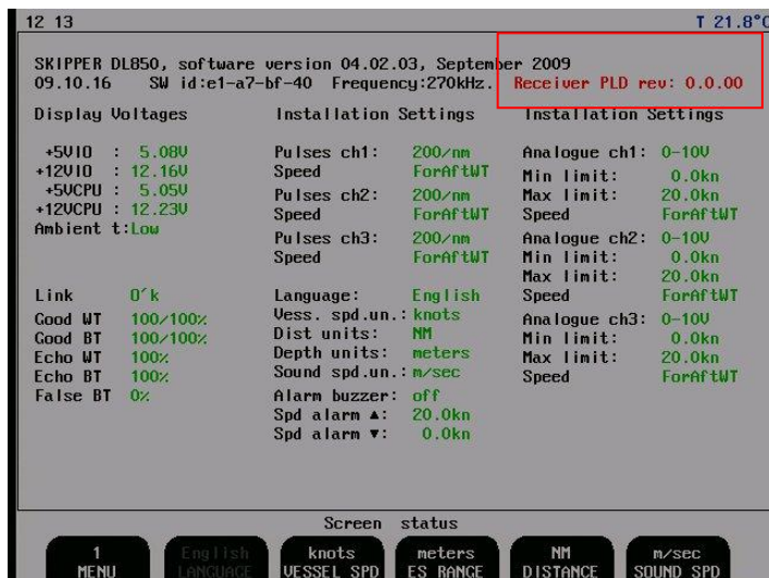
Status screen in new software with old PLD version 0.0.0 installed
